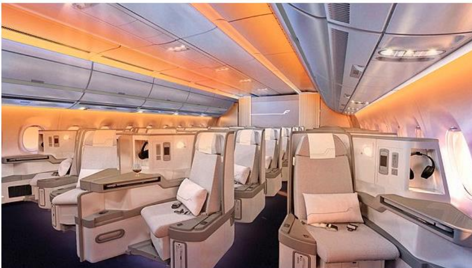
Inside the Business Class cabin, where atmospheric lighting mimics the time of day to help passengers adjust
